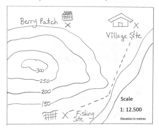
On this map the scale is 1:12,500. The first number in the "scale factor" is the distance on a map (or drawing) and the second number is the distance in real life.
