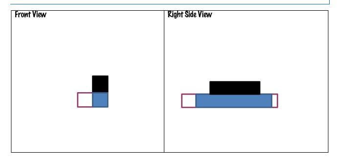
If the Left Side View is required, place the Left Side View in the lower left quadrant and the Front View in the lower right quadrant.
