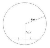
Demonstrate how to draw in the missing side to form a right triangle and use Pythagoras to determine the missing side. From there, simply multiply by 2 to determine the length of the chord. Therefore the length of the missing side is 4cm, and the entire chord length must be:
